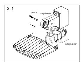
4.Refer to picture 4 using the machine screws secure the lamp holder.
