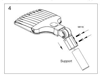
5.Refer to picture 5 locking bolt can be only compatible with a lamp pole that the outer diameter is  $\phi$ 60, lamp adjustable angle is 0-90°.
